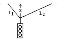
50. A 100 N traffic light is suspended by two wires of length  $L_1$  and  $L_2$  as shown in the figure. If  $L_1 = 3.0$ m and  $L_2 = 5.0$  m and the distance x = 2.0 m, then the tension in the wire of length  $L_1$  is, a. 125 N
