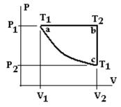
48. The PV diagram for one mole of an ideal gas is shown in the figure above. P1 = 3 atm, P2 = 1 atm, V1 = 7 liters, and V2 = 21 liters. What is the temperature T1 at point a?
